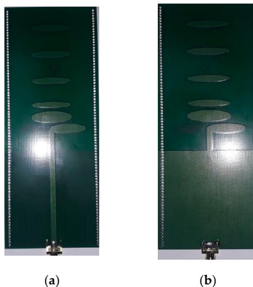
**Figure 6.** Photograph of the fabricated proposed antenna (a) front view (b) back view.
