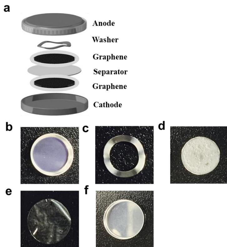
**Figure S3.** Structure of coin cell type supercapacitor. (a) schematic illustration of a coin cell type supercapacitor. (b) A photo of the anode. (c) Wave washer. (d) Graphene printed on the electrode. (e) Polymer electrolyte (PVA/H<sub>3</sub>PO<sub>4</sub>). (f) Cathode.
