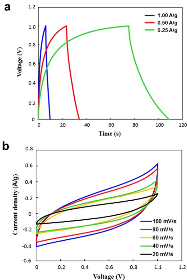
**Figure S4.** Properties of a two-electrode coin cell type supercapacitor. (a) Galvanostatic charge/discharge testing results at a current density from 0.25 to 1 A/g. (b) Cyclic voltammetry (CV) diagram with varying scan rate from 20 to 100 mV/s.
