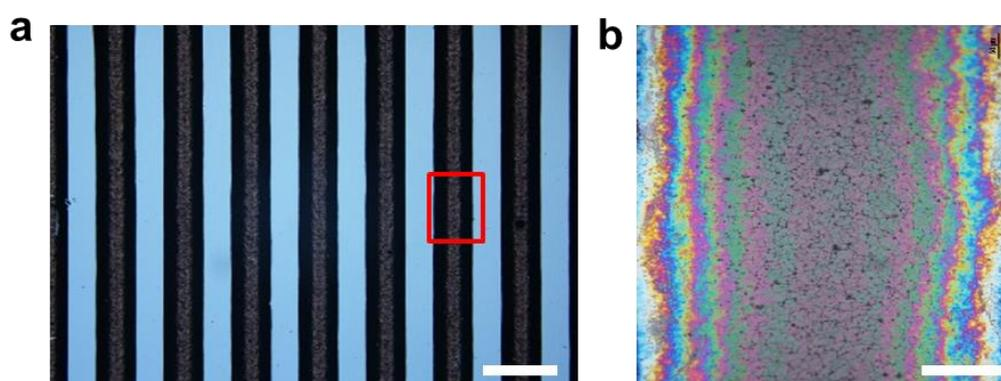
**Figure S2.** (a) EHD jet printed linear pattern. The scale bar is 500  $\mu\text{m}$ . (b) The magnification image in (a) shows the coffee ring effect. The color of the pattern is gradually changed by different of the GO thickness. The scale bar is 100  $\mu\text{m}$ .
