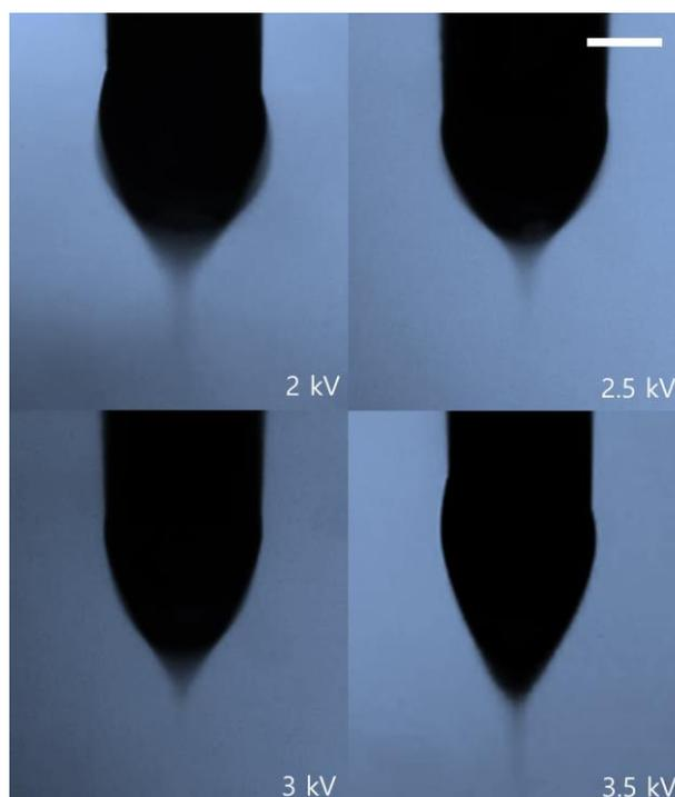
**Figure S1.** The effect of voltage on the thickness of the jet fiber. The scale bar is 100  $\mu\text{m}$ .
