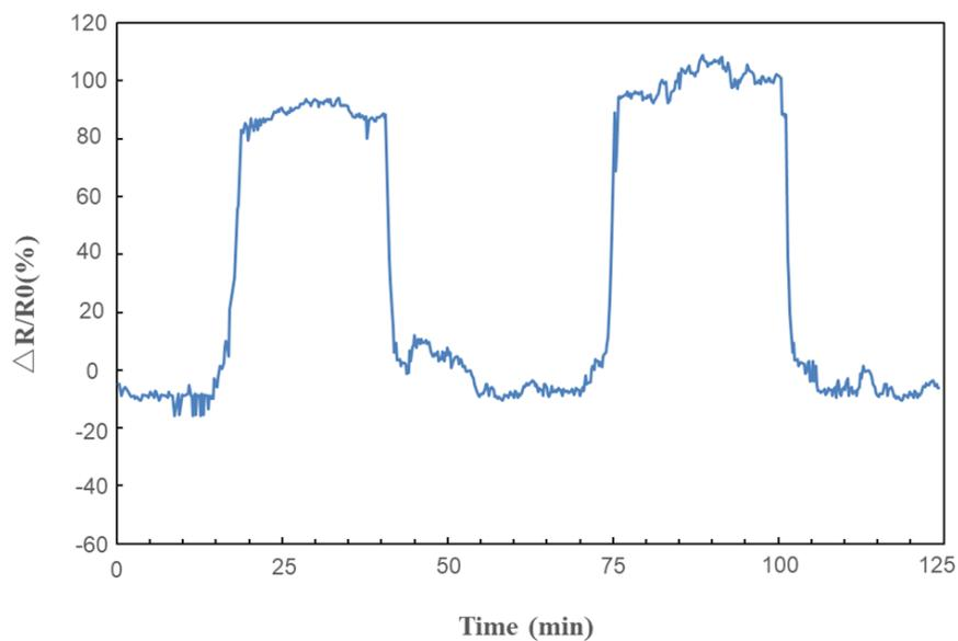
**Figure S5.** The saturation curve of the high aspect ratio sensor.
