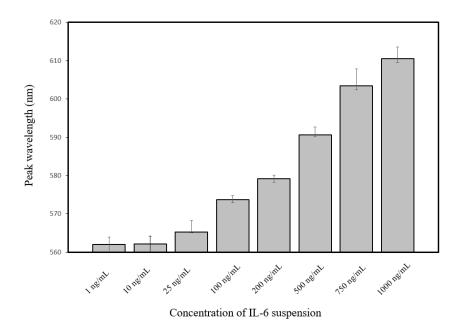
Figure S4. Calibration curve for concentrations 1 ng/mL, 10 ng/mL, 25 ng/mL, 100 ng/mL, 200 ng/mL, 500 ng/mL, 750 ng/mL and 1000 ng/mL IL-6 peak wavelength using fabricated plasmonic device in dry conditions (dry with pure  $N_2$  gas).
