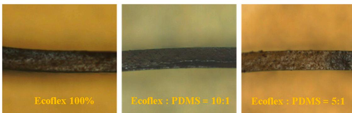
**Figure S4.** Cross-sectional images of the double elastomer layer according to the mixture ratio of Ecoflex and polydimethylsiloxane (PDMS).**Table S4.** Thickness of the double elastomer layer according to the mixture ratio of Ecoflex and polydimethylsiloxane (PDMS).
