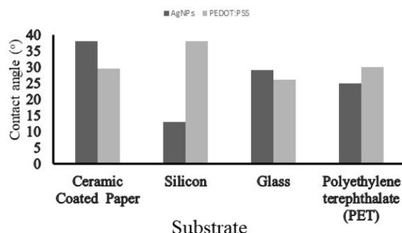
**Figure 2.** Contact angles measured via the sessile drop analysis method for the silver nanoparticles (AgNPs) and poly(3,4-ethylenedioxythiophene)-poly(styrenesulfonate) (PEDOT:PSS) inks and four potential substrates. The contact angle can be easily influenced by the nature of the substrate, mainly the surface.
