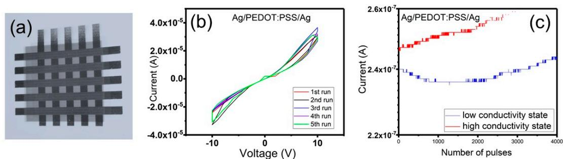
**Figure 9.** (a) Optical microscopy image of the printed crossbar memory cells. (b)  $I$ – $V$  characteristics of five consecutive runs of the Ag/PEDOT:PSS/Ag memory elements. (c) The memory retention time of the printed cells.
