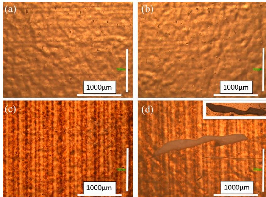
**Figure 7.** Optical microscopy images of the PEDOT:PSS ink pattern after one pass (a) before and (b) after removal of adhesive tape, and after five passes (c) before and (d) after removal of the adhesive tape.
