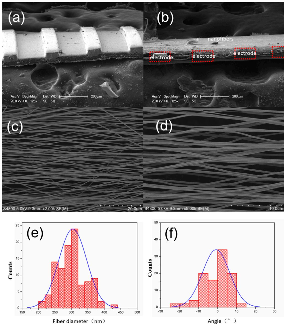
**Figure 2.** (a) SEM image of the flexible parallel copper electrode, (b) side view SEM image of the P(VDF-TrFE) nanofibers and electrode after electrospinning process, (c) top view SEM image of the nanofibers, (d) enlarged SEM image of the nanofibers, (e) typical fiber diameter distribution statistics, (f) fiber orientation distribution statistics.
