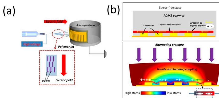
**Figure 3.** (a) Schematic of the electrospinning experimental setup. (b) Cross-sectional view of the generator.
