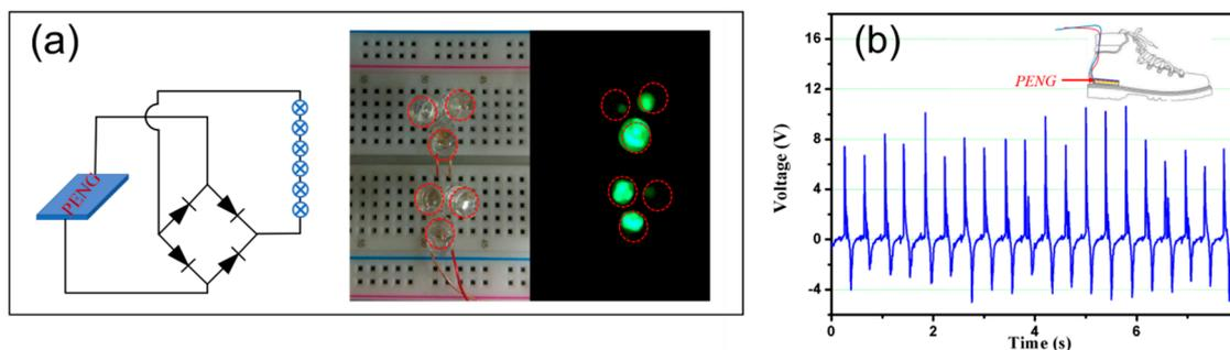
**Figure 5.** (a) The lighted LEDs and associated circuit diagram: (b) Output voltage generated by human walking.
