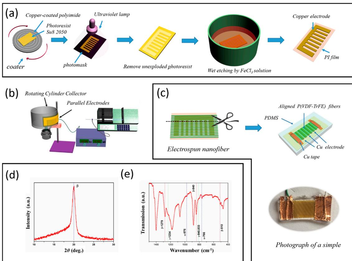
**Figure 1.** (a) Schematic diagram of flexible parallel copper electrode fabrication, (b) the schematic of electrospinning progress, (c) nanogenerator fabrication, (d) X-ray diffraction (XRD) pattern of the P(VDF-TrFE) nanofibers, (e) infrared spectra of the P(VDF-TrFE) nanofibers.
