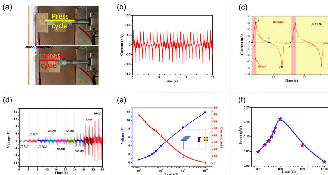
**Figure 4.** (a) Scheme of the press cycle and release cycle of mechanical loading equipment, (b) the short-circuit current of PENG during pressing–releasing cycles, (c) signal analysis corresponding to the cyclic pushing–releasing process, (d) output voltages from PENG with different load resistances, (e) the variation of output voltages and calculated currents across load resistances (inset is the corresponding circuit), (f) power density across different load resistances.
