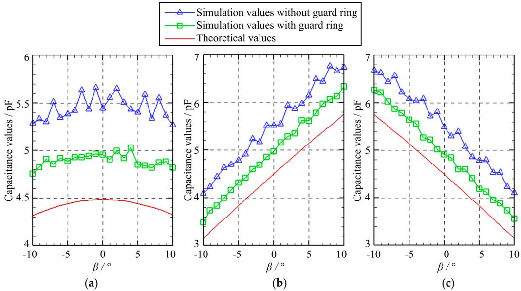
Figure 5. The capacitance variation of three capacitors in the case of A: (a)  $C_1$ ; (b)  $C_2$ ; (c)  $C_3$ .
