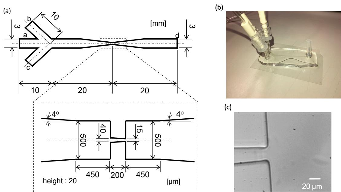
**Figure 1.** (a) Schematic drawing of the microflow channel—*a*, inlet port for cell flow; *b* and *c*, inlet ports for sheath flow; and *d*, outlet. (b) A fabricated microfluidic device and (c) a magnified view of the tip of the microflow channel.
