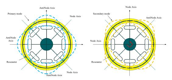
Figure 4. DUVRG resonant structure drive mode (left) and sense mode (right).
