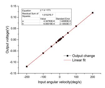
Figure 16. DUVRG scale factor test result.
