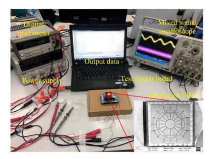
Figure 13. DUVRG bias and frequency test platform.
