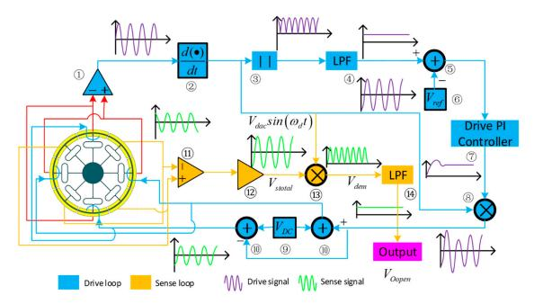
Figure 11. DUVRG system schematic diagram.
