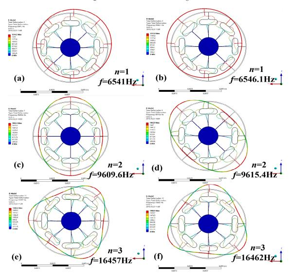
**Figure 7.** Modal diagram of the mode number n = 1, 2 and 3.
