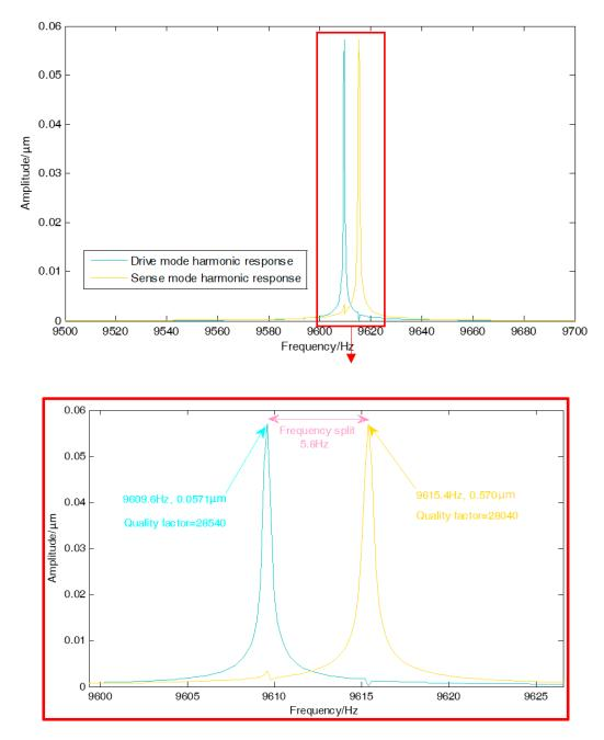
Figure 8. Amplitude frequency response curve of DUVRG.
