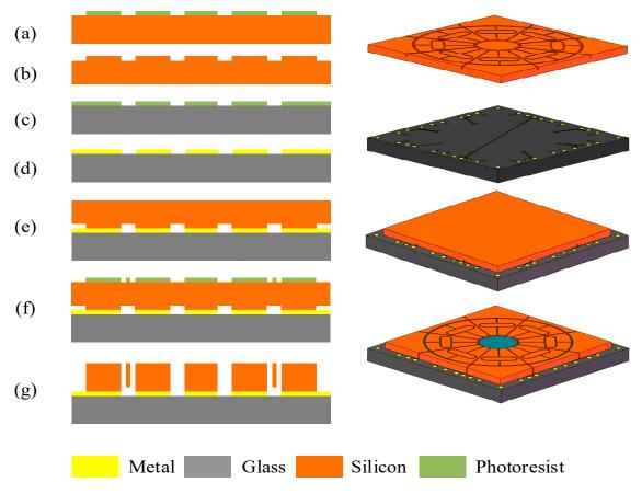
Figure 9. Main process flow of fabrication of DUVRG.
