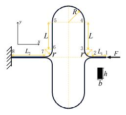
Figure 6. Double-U beam stiffness diagram.
