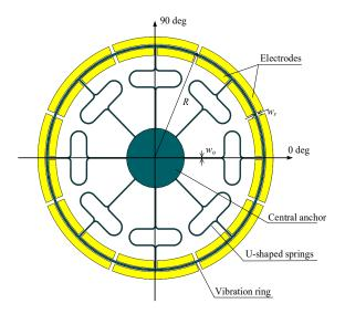
Figure 2. DUVRG resonant structure diagram.
