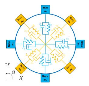
Figure 3. DUVRG resonant structure mechanical equivalent model.
