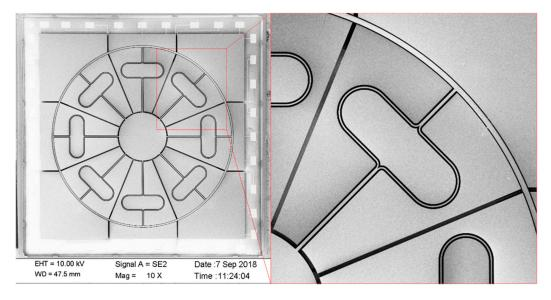
Figure 10. Scanning electron micrograph image of the fabricated DUVRG.
