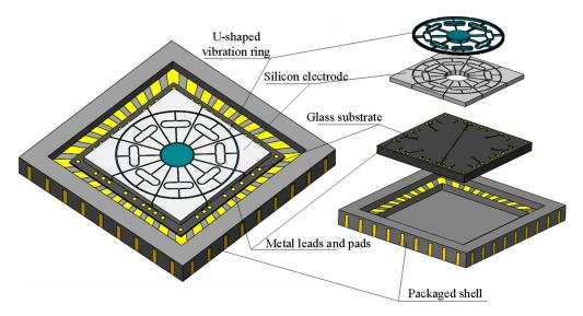
Figure 1. Double U-beam (DUVRG) structure chip diagram.
