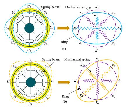
Figure 5. (a) DUVRG drive mode stiffness model. (b) DUVRG sense mode stiffness model.
