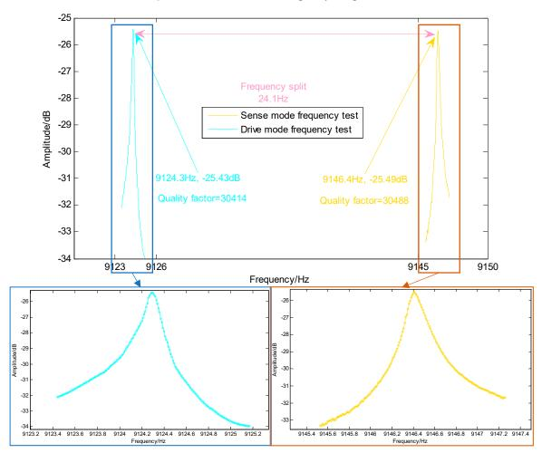
Figure 14. DUVRG structure frequency test results.
