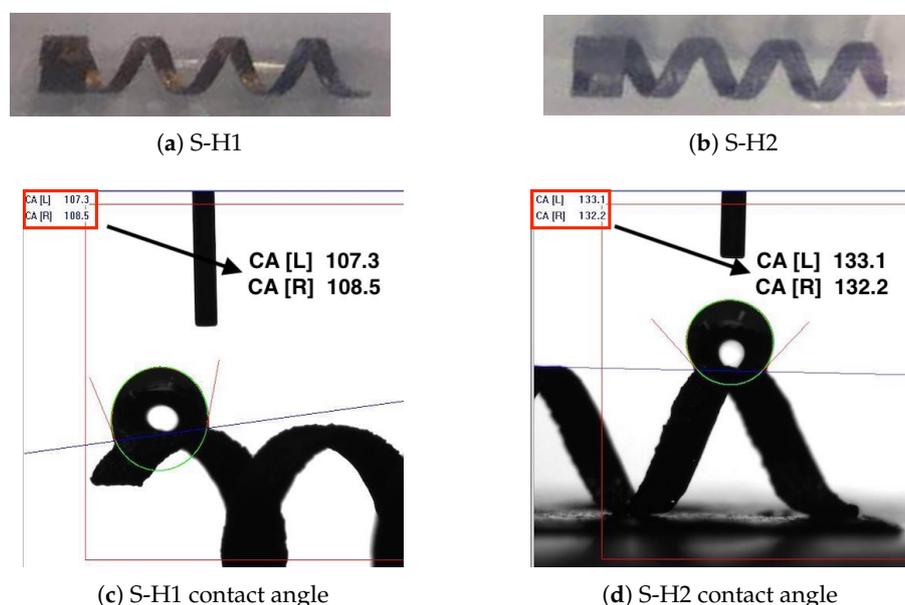
**Figure 3.** (a) S-H1: helical swimmer with less hydrophobic surface; (b) S-H2: helical swimmer with more hydrophobic surface. (c,d) The measured contact angles for S-H1 and S-H2.
