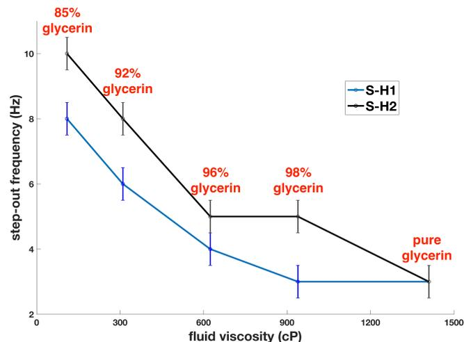
Figure 5. Step-out frequencies of S-H1 and S-H2 under increasing fluid viscosity.
