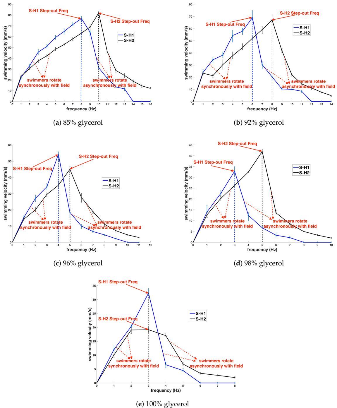
**Figure 4.** The propulsion velocity of S-H1 and S-H2 as a function of rotation frequency in different viscous liquids.
