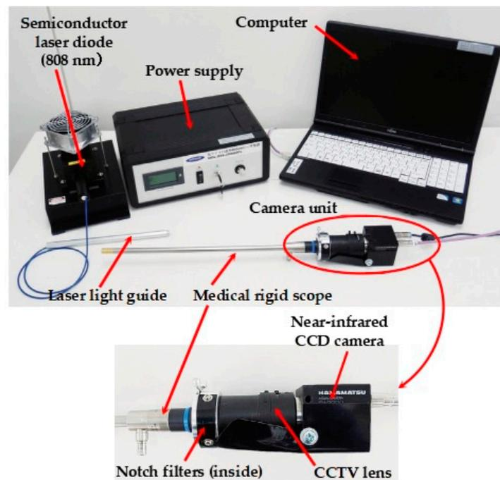
**Figure 4.** The laparoscopic fluorescent detection system composed of a medical rigid scope with a near-infrared CCD camera, a semiconductor laser diode (808 nm) as an excitation light source, and a computer with monitor.
