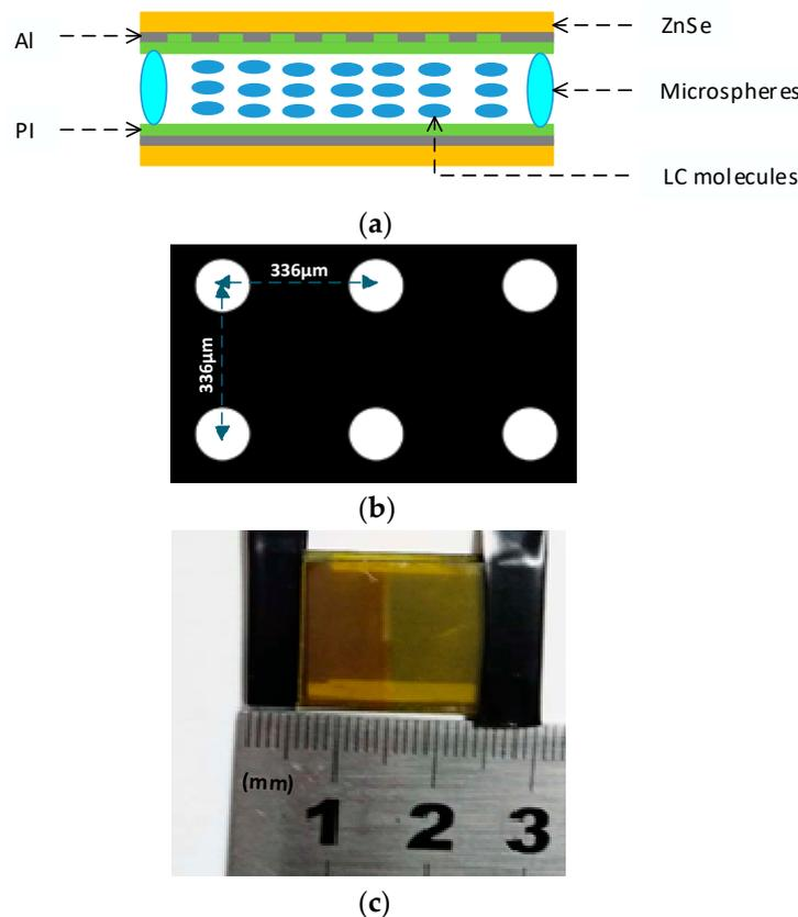
**Figure 1.** The dual-mode liquid-crystal (LC) micro-device—(a) main architecture; (b) patterned Al electrode; and (c) appearance of the final micro-device.
