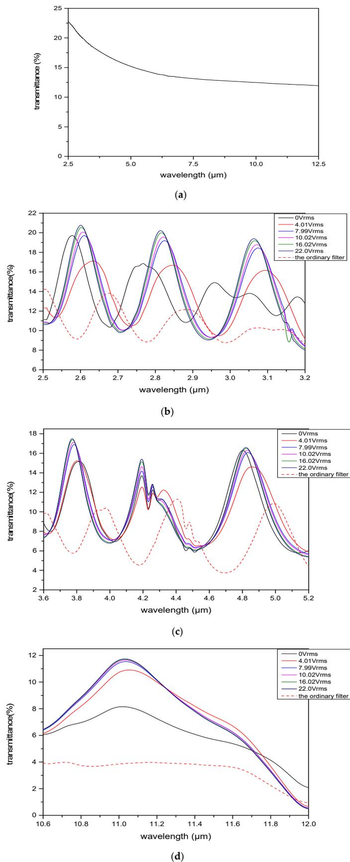
**Figure 2.** The results of spectral filtering showed the transmittance of (a) the substrate covered by Al film; (b) wavelength band from 2.5 to 3.2  $\mu\text{m}$ ; (c) wavelength band from 3.6 to 5.2  $\mu\text{m}$ ; and (d) wavelength band from 10.6 to 12.0  $\mu\text{m}$ . The signal voltages included were 0  $V_{\text{rms}}$ , 4.01  $V_{\text{rms}}$ , 7.99  $V_{\text{rms}}$ , 10.02  $V_{\text{rms}}$ , 16.02  $V_{\text{rms}}$ , and 22.00  $V_{\text{rms}}$ .
