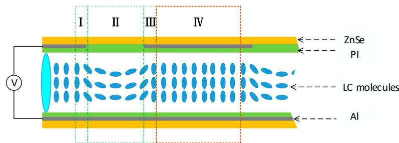
**Figure 6.** The cross-sectional view of the structural piece of the dual-mode LC micro-device.
