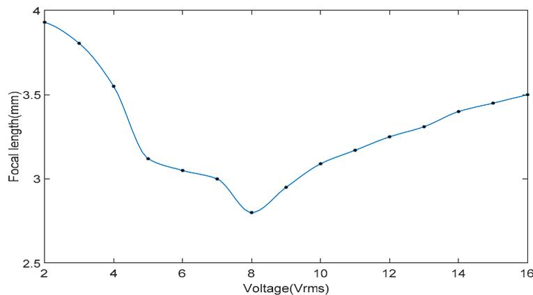
**Figure 5.** The relationship between the focal length of the dual-mode LC micro-device and the signal voltage applied.
