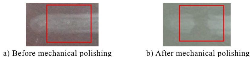
Figure 11. Photographs of APPP processed surface appearance before and after mechanical polishing.
