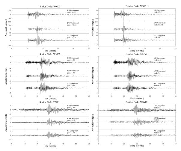
**Figure 5.** Examples of three-component accelerations from 31 October 2018, *M* 5.1 Xichang earthquake at the following co-located station pairs: W0107&51XCH, W3302&51MNJ, and T2405&51SMX. Stations 51XCH, 51MNJ, and 51SMX are traditional strong-motion stations with trigger-mode data transmission.
