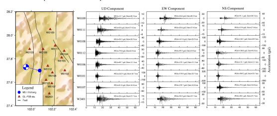
**Figure 8.** A series of acceleration waveforms recorded by GL-P2B sensor network during the 31 October 2018, *M* 5.1 Xichang earthquake. These plots show the data quality of the network for up–down (UD), east–west (EW), and north–south (NS) components.
