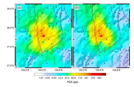
**Figure 7.** PGA shake maps for the 16 May 2018, *M* 4.3 Shimian earthquake (**a**) with and (**b**) without virtual stations. PGA values for the virtual stations were derived using the ground-motion prediction equation proposed in Yu's study [41]. The triangles represent the GL-P2B stations, while the star indicates the epicenter of this earthquake.
