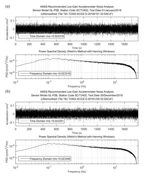
**Figure 4.** An example of noise data of the sensor SC/T2402 processed by a Butterworth bandpass filter between 0.1–20 Hz and the computed root mean square (RMS), power spectral density (PSD) values: (a) Results of the noise data obtained on 1 January 2018; (b) results of the noise data obtained on 30 December 2018.
