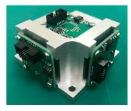
**Figure 2.** Photo of the Micro Electro Mechanical System (MEMS) acceleration sensor, in which three MSV6000-02 accelerometers are mounted orthogonally to each other.
