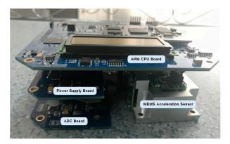
Figure 1. Hardware components of GL-P2B.
