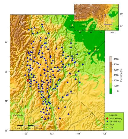
**Figure 3.** Station distribution of the GL-P2B based seismic sensor array shown as blue triangles. The red circle represents the epicenter of the 31 October 2018, *M* 5.1 Xichang earthquake. A large map with the marked study region is shown in the inset. Black lines indicate faults reported by Deng's research [39].
