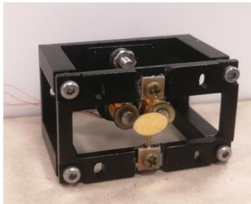
Figure 4. Prototype of the external electromagnet FPCB micromirror.
