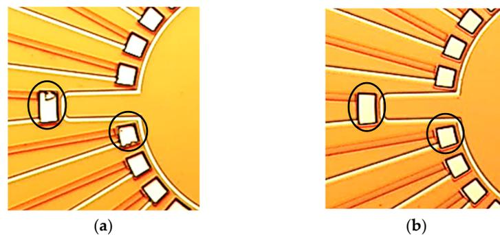
**Figure 7.** The condition of the structures (a) after the standard wet chemical etching by ‘TiW etch 100’ solution, residue left; (b) after the wet chemical etching in ‘TiW etch 100’ solution and a deep etching in the photoresist developer AZ 400K, perfectly cleaned.
