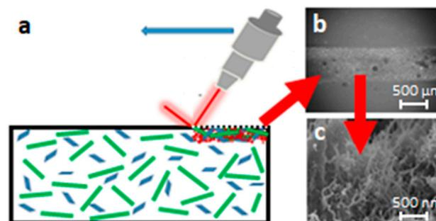
**Figure 1.** Effect of laser ablation on the surface (a); SEM micrographs at different magnifications of resulting tracks showing increased content of conductive filler (b,c).
