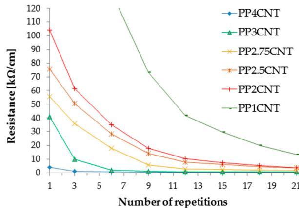
**Figure 3.** Decrease in track resistance with the number of laser treatments performed on polypropylene–ethylene copolymer (PP)/carbon nanotube (CNT) composites ( $P = 35\%$ , scan rate = 200 mm/s,  $F = 15$  kHz, defocus = 0 mm).
