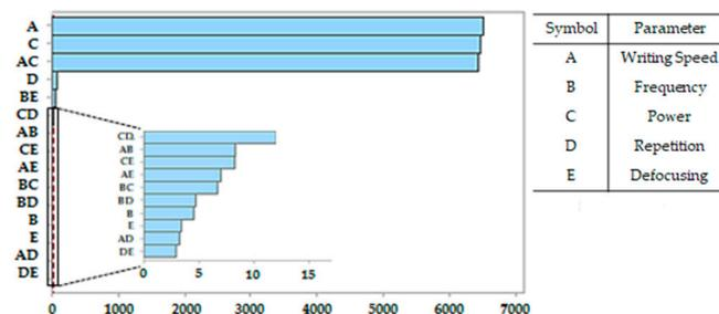
**Figure 2.** Pareto plot showing the relevance of different parameters and their combinations on the conductivity of tracks.
