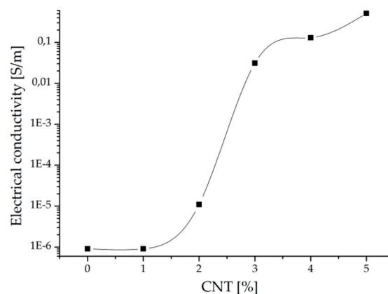
**Figure 5.** Percolation curve for ethylene–propylene–diene monomer (EPDM)/PP/CNT composites.
