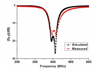
**Figure 6.** Measured and simulated  $|S_{11}|$  of the proposed implantable antenna.
