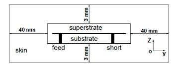
Figure 2. Side view of simulation model for the proposed implantable antenna.
