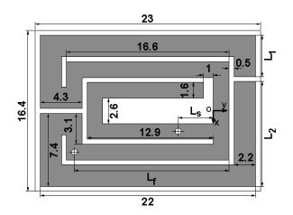
Figure 1. Geometry of the proposed implantable antenna (unit: mm).
