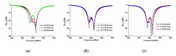
**Figure 4.** Comparison of  $|S_{11}|$  of the proposed antenna with different geometric parameters: (**a**) short position  $L_s$ ; (**b**) feed position  $L_f$ ; and (**c**) tuned strip length  $L_1$ .
