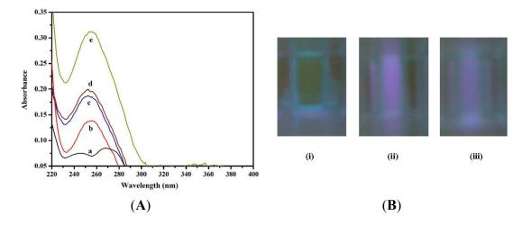
**Figure 2.** (**A**) UV absorption spectra of (a) TiO<sub>2</sub>; (b) Aptamer; (c) Aptamer-target complex (in absence of TiO<sub>2</sub>); (d) Aptamer-target complex (in presence of TiO<sub>2</sub>); and (e) Aptamer-TiO<sub>2</sub> complex; (**B**) Fluorescence imaging of (i) FAM-aptamer; (ii) aptamer-TiO<sub>2</sub>; and (iii) aptamer-target complex (in presence of TiO<sub>2</sub>).
