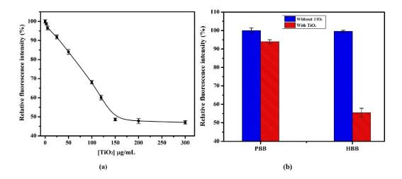
**Figure 3.** (a) Quenching effect of TiO<sub>2</sub> on fluorescence intensity of FAM-labeled aptamer (final concentration 2.0  $\mu$ M) in HBB at pH 7.4; (b) Effect of HBB and PBB at pH 7.4 on quenching performance of TiO<sub>2</sub> (final concentration, 150  $\mu$ g/mL). The error bars were obtained from three parallel experiments.
