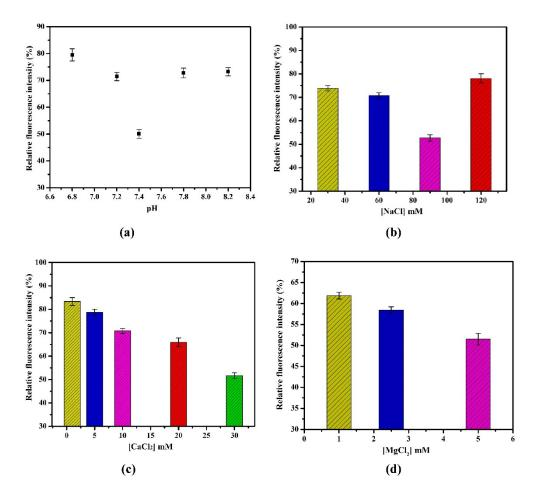
**Figure 4.** (a) Effect of pH (6.8–8.2) in HBB on quenching performance of TiO<sub>2</sub>; (b) Effect of NaCl concentrations (30, 60, 90 and 120 mM) on quenching performance of TiO<sub>2</sub>; (c) Effect of CaCl<sub>2</sub> concentrations (1, 5, 10, 20 and 30 mM) on quenching performance of TiO<sub>2</sub>; (d) Effect of MgCl<sub>2</sub> concentrations (1, 2.5 and 5 mM) on quenching performance of TiO<sub>2</sub>. The error bars were obtained from three parallel measurements.
