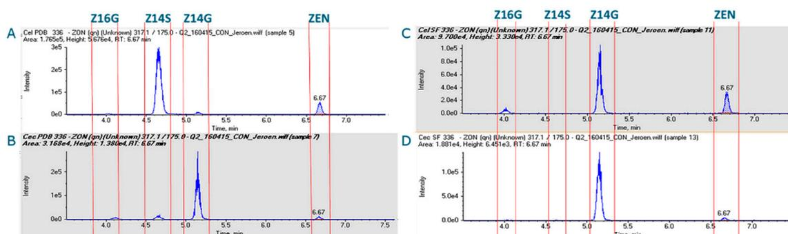
**Figure 2.** LC-MS/MS chromatograms ( $m/z$  317.1→175.0) for the production of Z14G, Z16G and Z14S metabolites by *Cunninghamella elegans* in PDB medium (A) and synthetic depletion medium (C) and *Cunninghamella echinulata* in PDB medium (B) and synthetic depletion medium (D).
