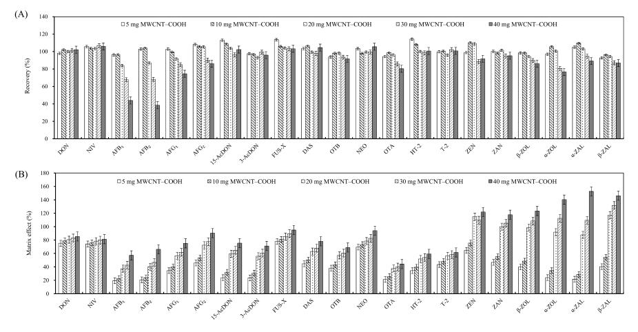
**Figure 3.** Effects of different amounts of MWCNT–COOH and 200 mg C<sub>18</sub> on the recovery and matrix effect of mycotoxins in corn. Vertical bar represents  $\pm$  standard error (*n* = 3). (**A**) Recovery (%); (**B**) Matrix effect (%).
