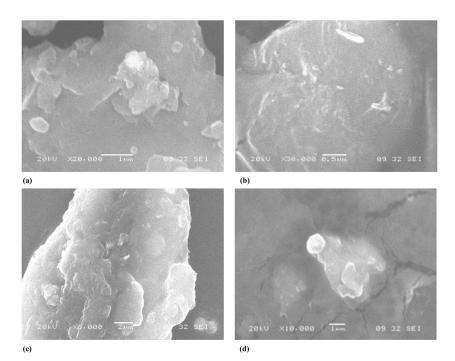
**Figure 3.** Scanning electron microscope (SEM) images of forest honey (**a**) and AgNPs synthesized using 20% (**b**), 40% (**c**), and 80% forest honey (**d**).
