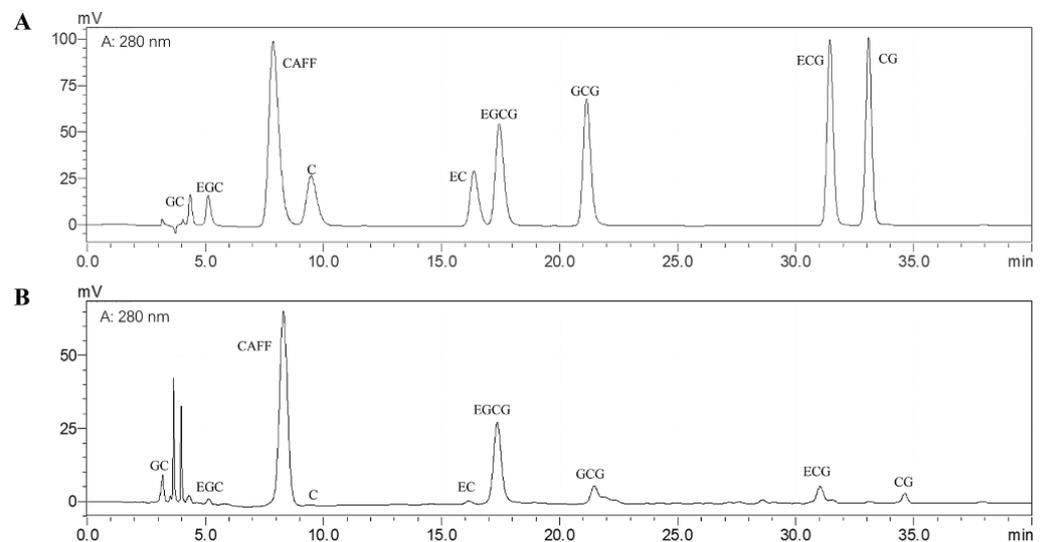
**Figure 1.** The UPLC chromatograms of catechin monomers and caffeine in the matcha sample. (A) Standard mixture; (B) matcha sample.
