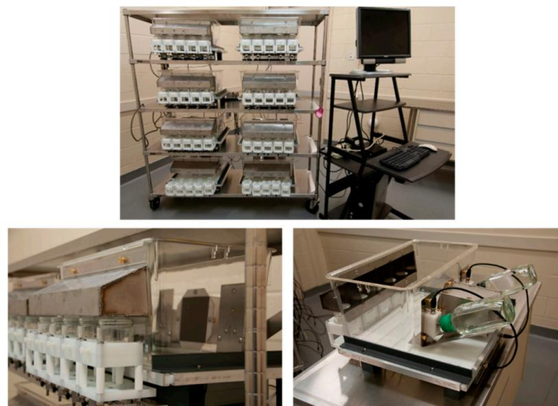
**Figure 1.** The five-Item Food Choice Monitor. Top: a set of customized cages connected to a computer. Bottom left: the front of a single cage, showing the components to measure food intake—the stainless-steel food hood, glass jars, HDPE jar holders and load cells to measure food intake. Bottom right: the back of a single cage, with the stainless-steel nest flanked by bottles set into the lick blocks, connected by cable to the interface box under the base of the unit.
