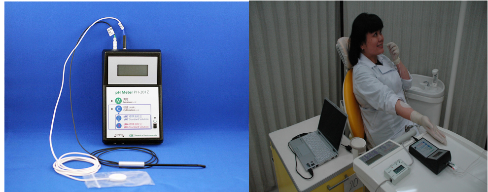
Figure 1. Measurement of enamel surface pH [13]. Left: pH antimony electrode connected to pH meter. Right: Photograph taken during enamel surface pH measurement.
