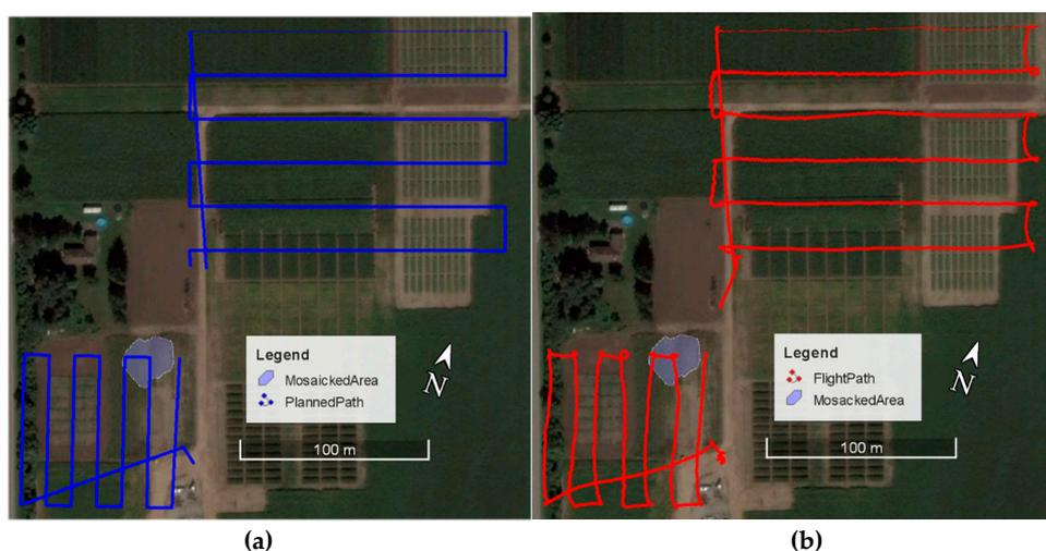
**Figure 3.** The study site with the planned flight path (a), and the actual flight path (b) draped over a Google Earth image, taken on a later date (3 September 2016). (Site 1 at bottom left: tomato field; Site 2 in upper right: corn and soybean fields).
