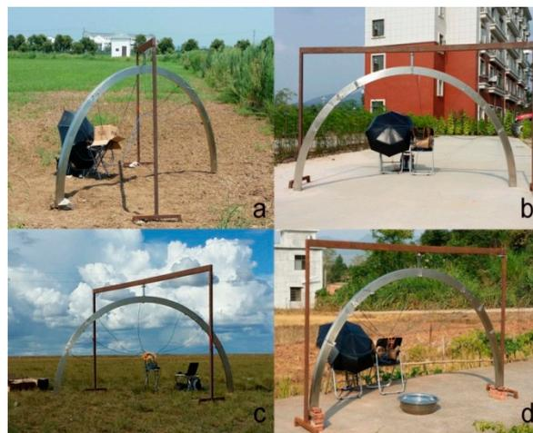
**Figure 3.** Radiant surface temperature (RST) observation experiments over four typical surfaces: (a) bare soil in Nanjing, 2 August 2015; (b) concrete in Jiangmen, 29 October 2015; (c) grass in Xilinguole, 31 August 2015; and (d) water in Yongzhou, 25 October 2015.
