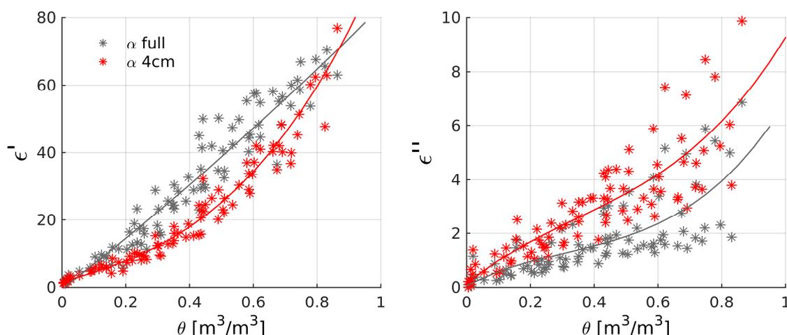
**Figure 3.** Estimated permittivities, (a) real  $\epsilon'$  and (b) imaginary  $\epsilon''$  part, of all organic samples measured over the entire wetness range  $\theta$  and at room temperature (filtered as specified in Section 2.2.3), using a filling factor  $\alpha$  for the full tube length (grey) and specifically calibrated for the 4 cm tube insertion depth (red).
