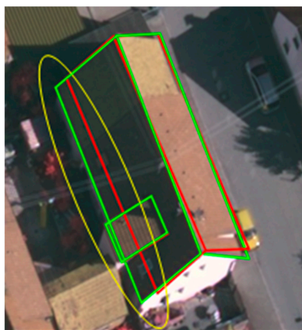
Figure 4. Matching line pair (marked in yellow) detected with increasing matching threshold; ALS-based lines (red), image-based lines (green).
