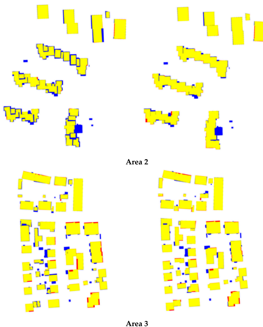
Figure 10. Qualitative assessment per-pixel level: buildings before ( left ) and after correction ( right ) (yellow: True Positive, blue: False Negative, red: False Positive).
