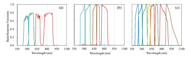
**Figure 1.** Band response functions for: FORMOSAT-2 (**a**); RapidEye (**b**); and WorldView-2 (**c**) satellite sensors used in this study.
