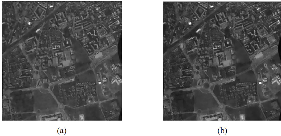
Figure 2. Edge preservation of guided filter: (a) Initial de-noised image; (b) Final de-noised image by guided filter.
