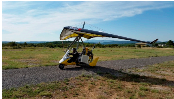
Figure 2. Tanarg 912 S BioniX 15 ultra-light aircraft (ULA). The airborne Lidar for atmospheric surveys using Raman Scattering (LAASURS) is embedded on the left side of the ULA.
