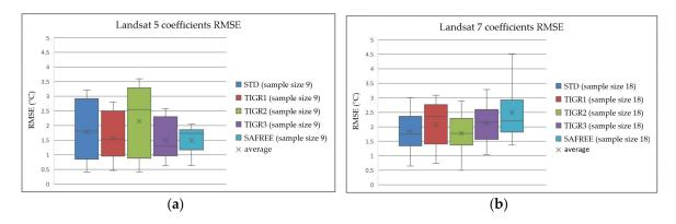
**Figure 2.** LST RMSE (root mean square error) boxplots for each coefficient table, where  $\times$  is the average, and the horizontal line inside box is the median. (a) Landsat 5 RMSE boxplots for each coefficient table calculated from all three available Landsat 5 delivered reference data; (b) Landsat 7 RMSE boxplots for each coefficient table calculated from all six ASTER reference images.
