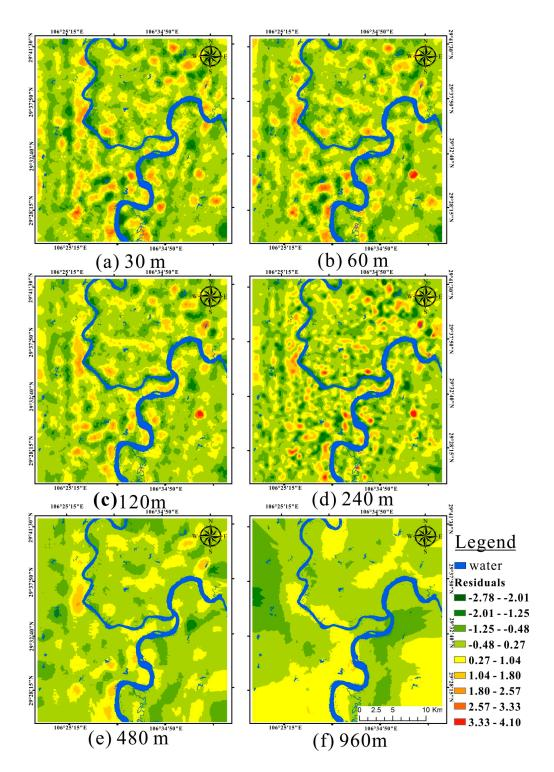
**Figure 6.** The spatial distribution of the local residuals in the multi-factor GWR models (using the SAVI, IBI, and NDSI as the explanatory variables simultaneously) at different spatial resolutions; (a)–(f) represent the spatial resolutions of 30 m, 60 m, 120 m, 240 m, 480 m, and 960 m, respectively. Moreover, the blue area represents water.
