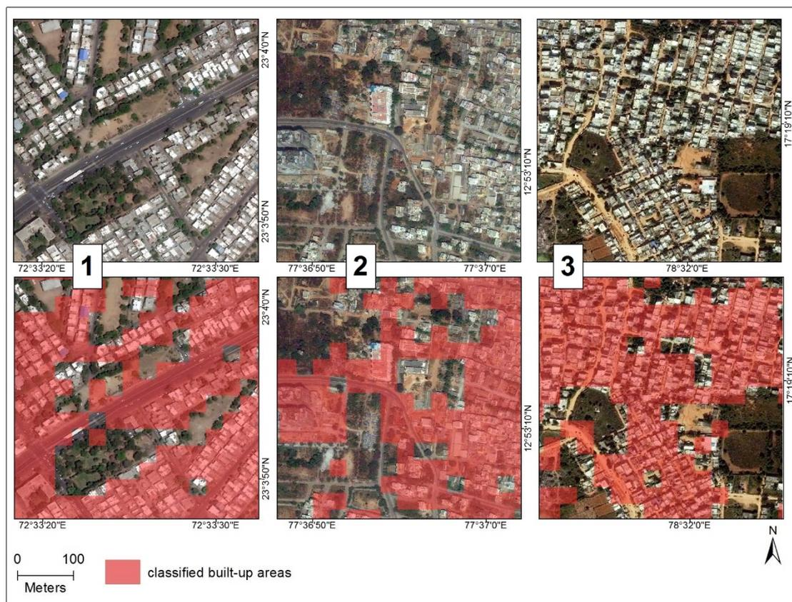
**Figure 12.** A detailed examination of the classification of built-up areas (visualized in red) compared to raw satellite images in five regions in India (classifier: Random forest with 10 trees, input: Landsat 8). Satellite images from DigitalGlobe. Includes copyrighted material of DigitalGlobe, Inc., All Rights Reserved.
