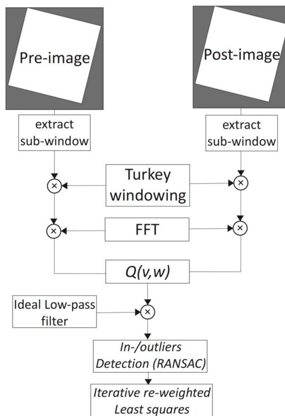
**Figure S2.** Algorithm workflow diagram of the applied robust phase fitting image cross-correlation method.
