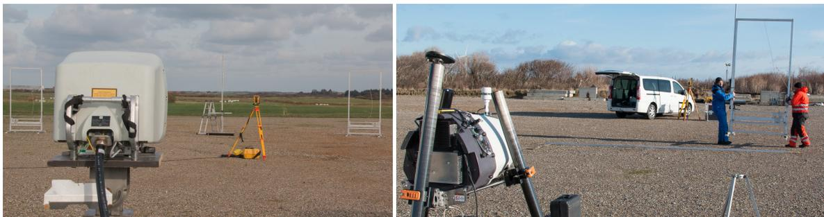
**Figure 4.** Field testing of the 5B (left) and ZDM (right): inclinometers calibration and beam trajectory verification.
