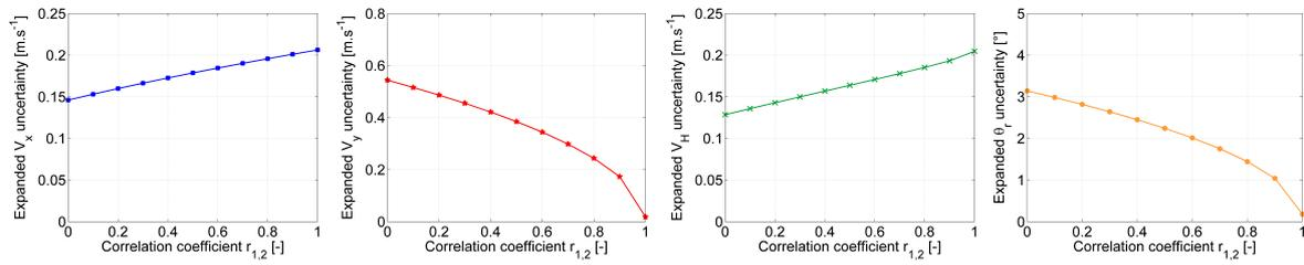
**Figure 12.** Expanded uncertainties  $U_{V_x}$ ,  $U_{V_y}$ ,  $U_{V_H}$  and  $U_{\theta_r}$  as a function of correlation coefficient  $r_{1,2}$  ( $V_H = 10 \text{ m}\cdot\text{s}^{-1}$ ,  $\theta_r = 5^\circ$ ,  $r_{xy} = 0.2$ ).
