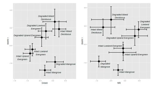
**Figure 4.** Normalized Top of Atmosphere Reflectance (TOA) of training data by forest type. Points indicate mean values while error bars depict upper and lower quartiles for Landsat 8 bands 3 (green), 5 (near infrared), and 6 (shortwave infrared 1). For each band, normalized reflectance was calculated by subtracting the mean and dividing by the standard deviation of the training data sample.
