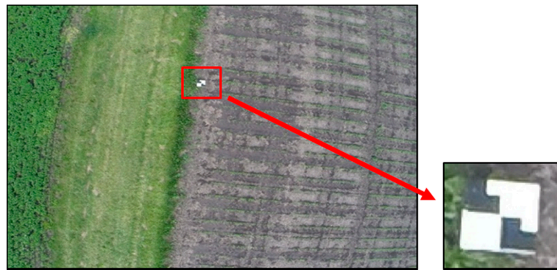
Figure 9. Sample RGB image over the test field with a close-up of one of the targets.
