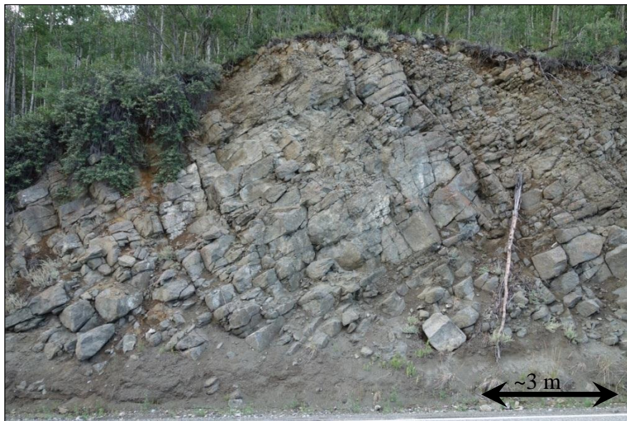
Figure 7. Photograph of rock slope study Site A showing three well-defined discontinuity sets.
