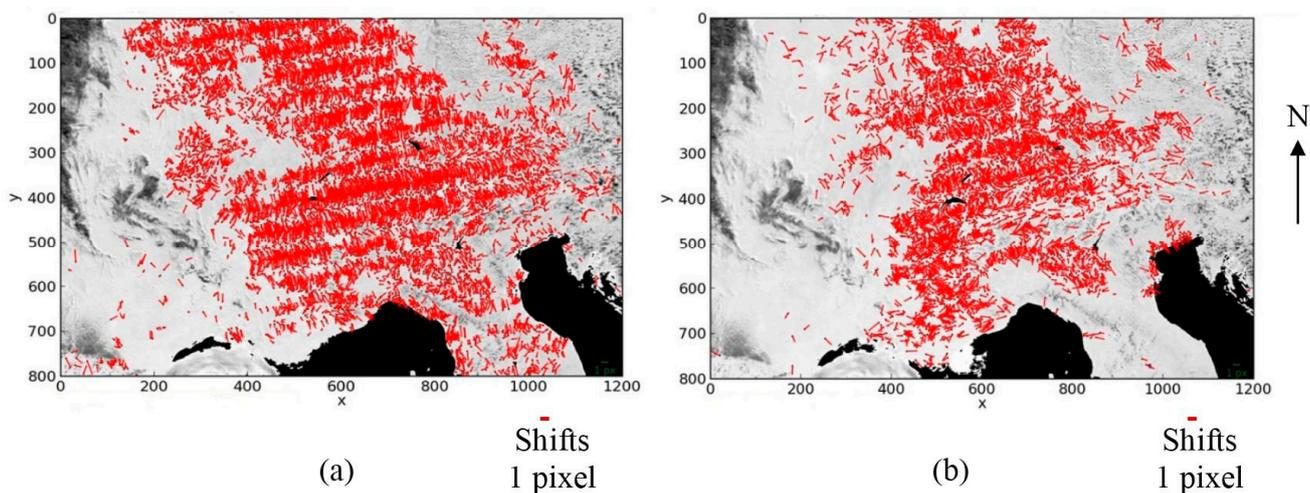
**Figure 12.** Image space shifts obtained from matching of NOAA-18-NOAA-19 (a) and NOAA-17-NOAA-19 (b) images acquired on 6 August 2009. The axes denote the image coordinates.
