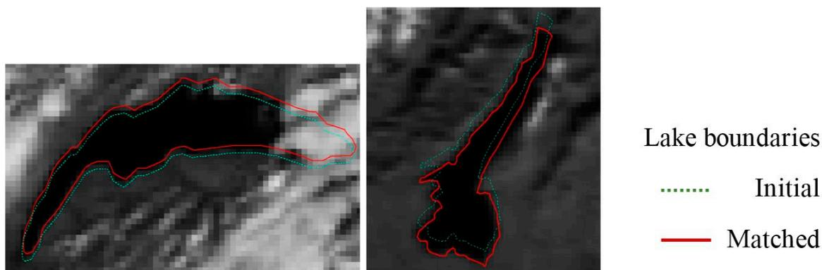
**Figure 15.** Lake matching results from Lake Lemman in a NOAA-17 image (**left**) and Lake Garda in a Metop-A image (**right**). The green polygons represent the initial positions of the lake points and the red polygons represent the matched positions.
