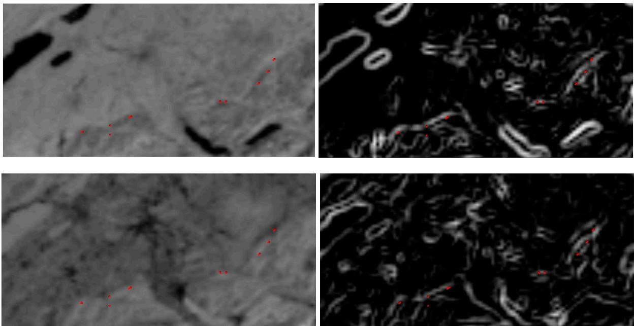
**Figure 6.** Parts of AVHRR Band-2 (**top**) and Band-5 (**bottom**) images acquired on 10 July 2008 at 09:36 from Metop-A. The matched points between the preprocessed images (**right**) are shown in both and presented on linear stretched images (**left**) as well.
