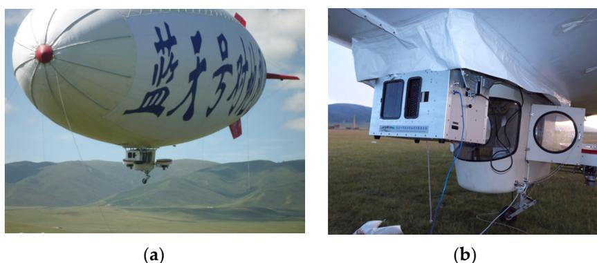
**Figure 1.** (a) “LanTianHao” HAA navigated at an altitude above 4100 m with a payload greater than 200 kg; and (b) docking of “LanTianHao” HAA and “LanTianHao” EOPS.
