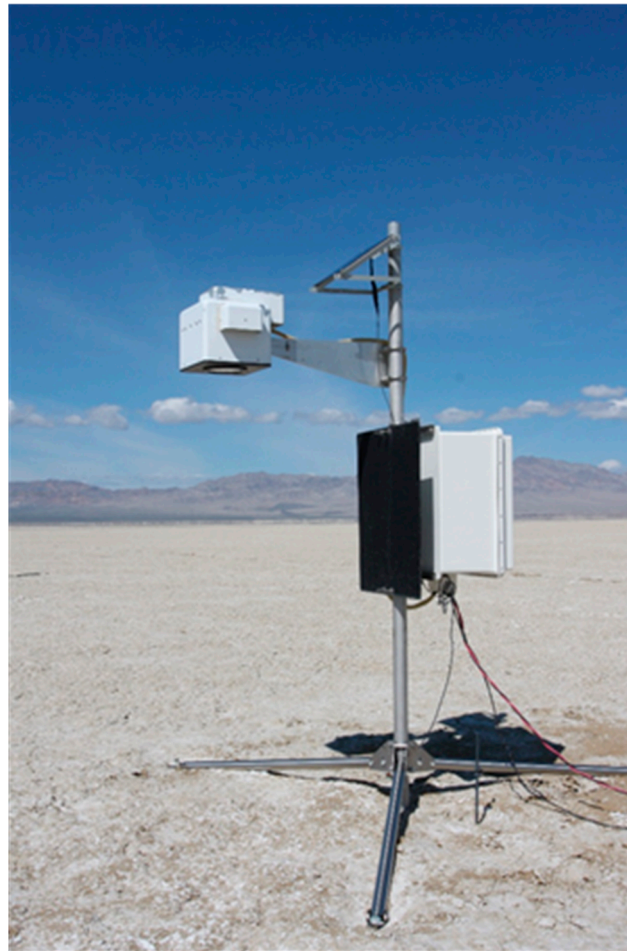
Figure 5. A ground-viewing radiometer at RadCaTS. The instrument head is 1.5 m above the surface. At this height, each of the eight detectors is viewing the same approximate area on the ground.
