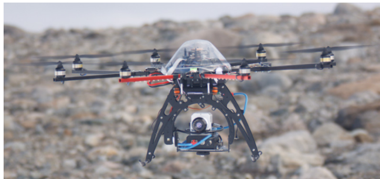
Figure 2. Oktokopter fitted with FLIR Photon 320 Thermal Infrared camera with Ethernet module mounted below.
