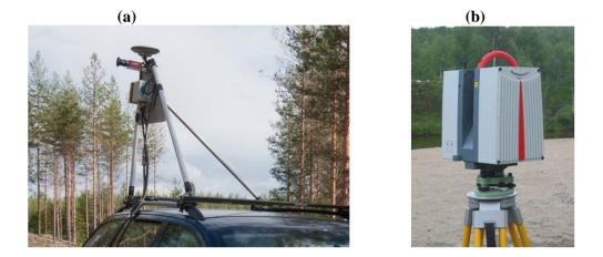
Figure 1. (a) The Sensei VLS system. (b) The Leica HDS6000 TLS system.
