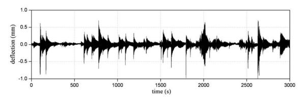
Figure 8. Deflection time-history measured by the radar sensor on the stay-cable  $S_{2U}$ .
