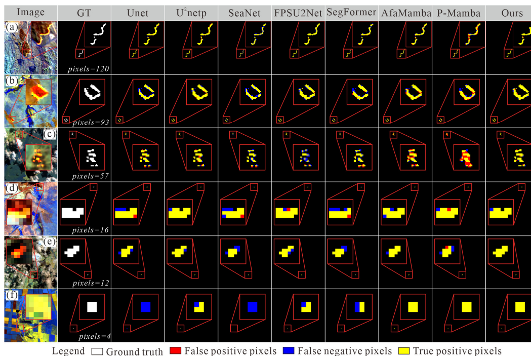
Figure 6. Visualization of segmentation results for fire points at different scales on the Oceania dataset. (a–f) represent six fire point samples with increasing scales.
