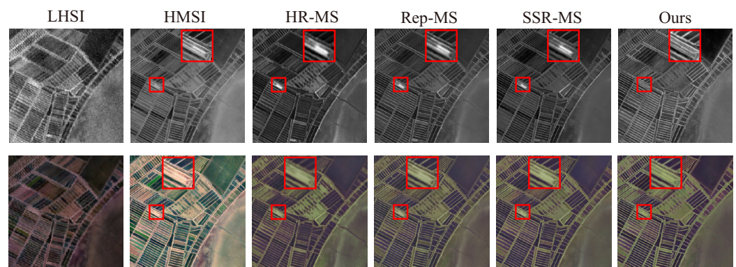
Figure 6. Original images and spectral enhancement results on GaoFen-5. The second band and false-color images (R:50, G:35, B:25 for LHSI and S^2R results; R:3, G:2, B:1 for HMSI) are placed from top to bottom in sequence. The red squares indicate the zoomed-in regions.
