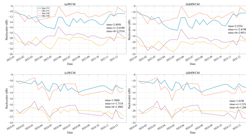
Figure 10. A comparison of simulated and Sentinel-1-observed backscattering at Canizal. (a) WCM simulation results in 2023; (b) MWCM simulation results in 2023; (c) WCM simulation results in 2024; (d) MWCM simulation results in 2024.
