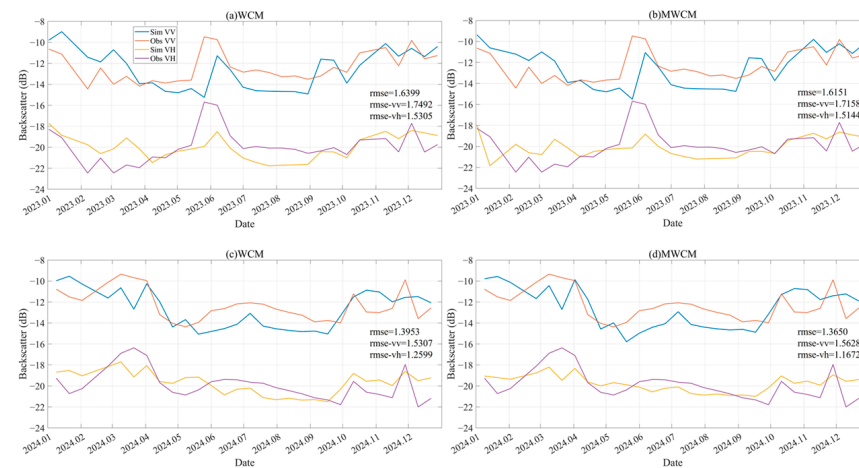
Figure 11. A comparison of simulated and Sentinel-1-observed backscattering at Zamarron. (a) WCM simulation results in 2023; (b) MWCM simulation results in 2023; (c) WCM simulation results in 2024; (d) MWCM simulation results in 2024.
