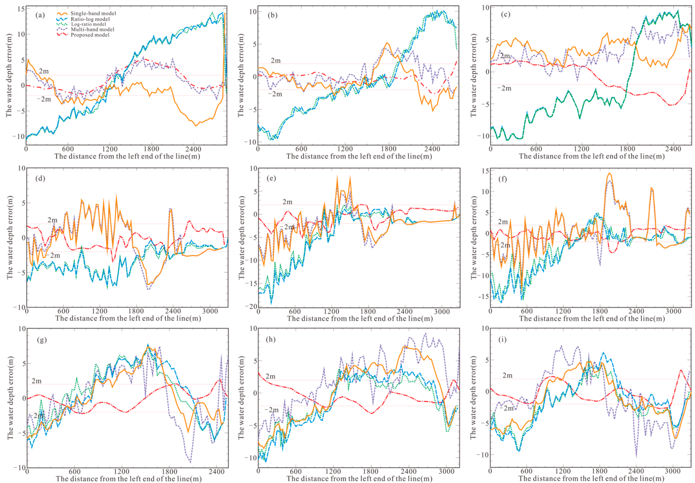
Figure 10. Verification of single-band model, ratio-log model, log-ratio model, multi-band model, and proposed model using check lines 1, 2, and 3 for Weizhou Island (a–c); Saipan Island (d–f); and Molokai Island (g–i).
